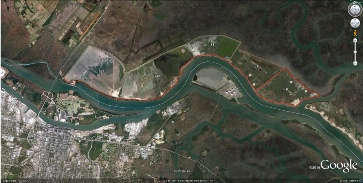
Figure 1. Dredge material containment areas (DMCAs) associated with the Savannah Harbor Expansion Project.
