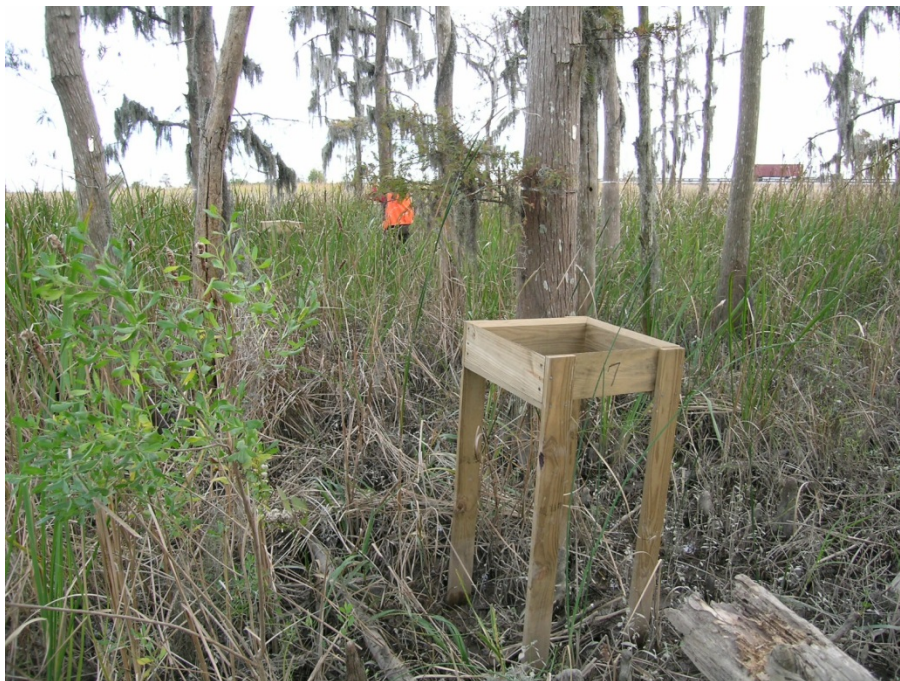
Figure 2. An example of a litter trap used to collect falling leaves, twigs, etc. The site depicted is not one being monitored as part of the SHEP.
