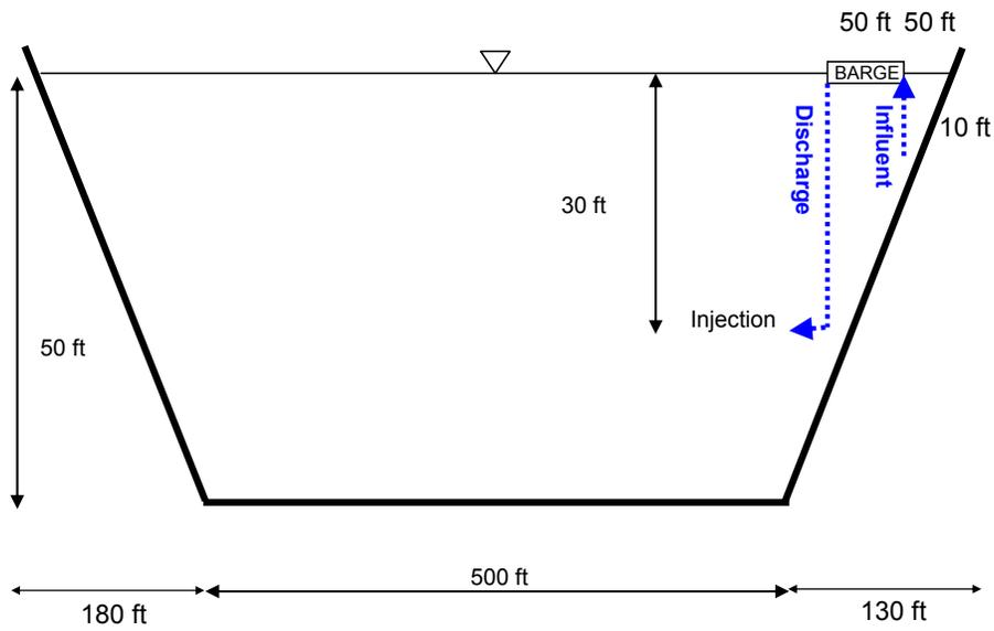
**Figure 1** Schematic of GPA dissolved oxygen injection experiment
