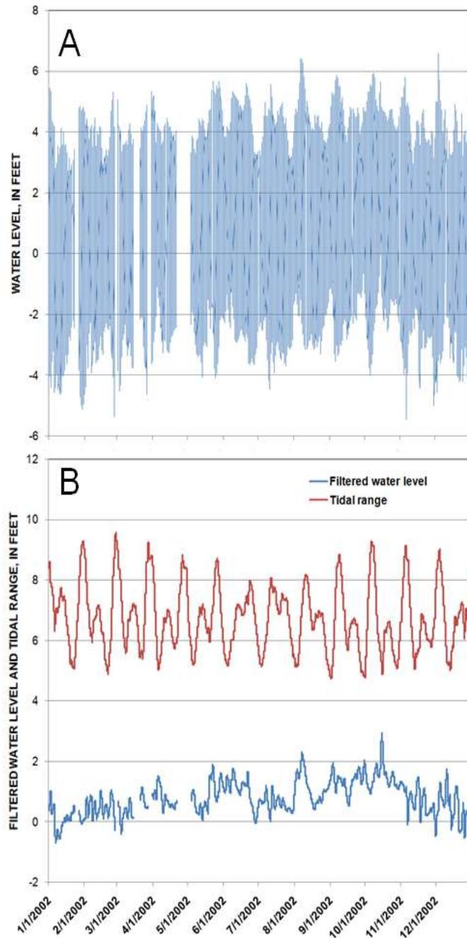
**Figure 3. Decomposition of the Fort Pulaski (station 02198980) 15-minute water-level signal (A) into the periodic component of tidal range and the chaotic component of daily water level (B).**
