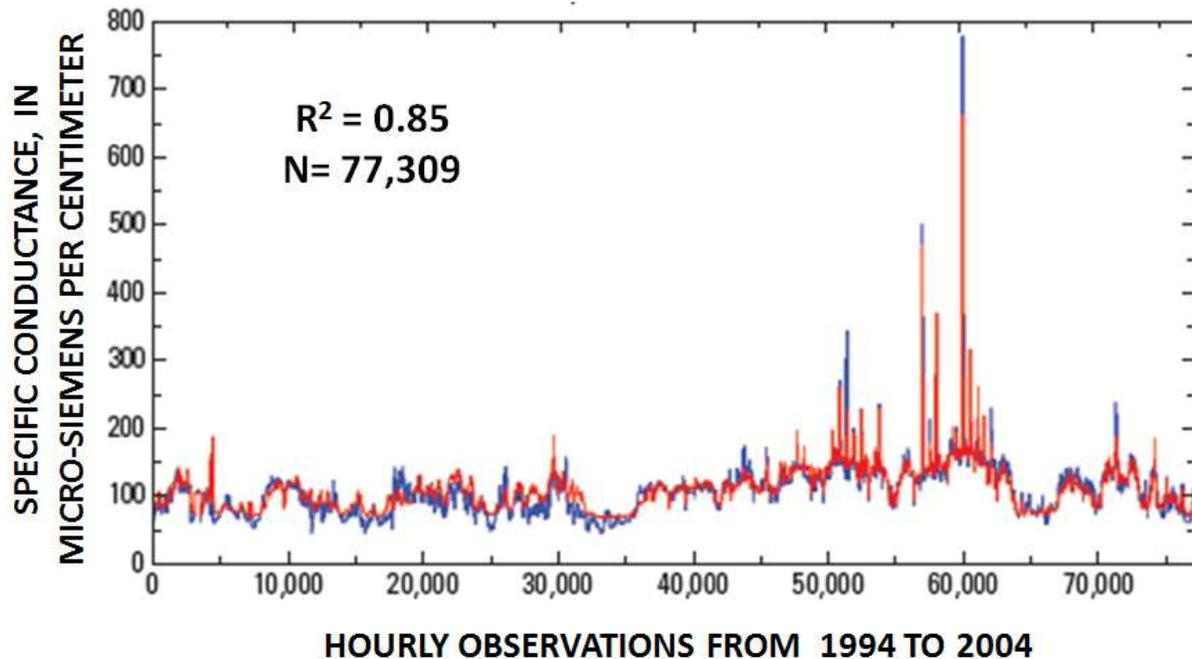
**Figure 4. Measured (blue trace) and predicted (red trace) daily specific conductance for the Savannah River at I-95 (station 02198840).**
