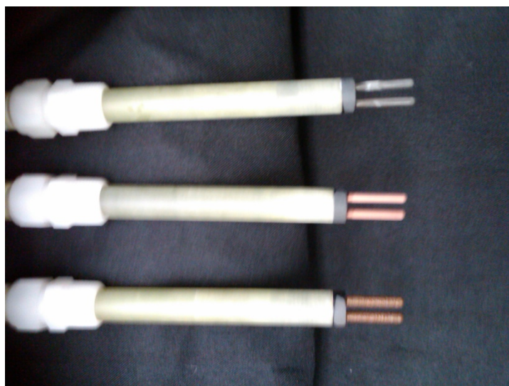
Photograph 3. Corrator® probes with steel, copper and lead electrodes.
