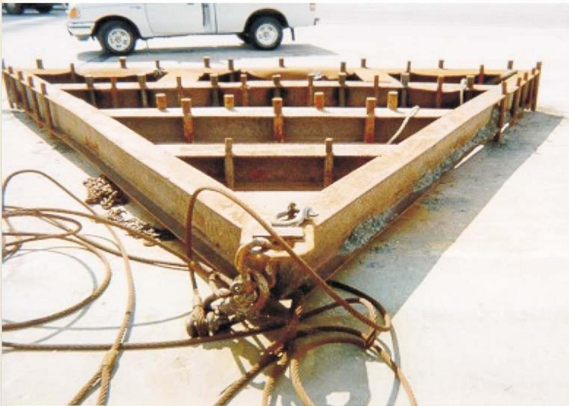
**Figure 1. I-beam agitation dredge.**
