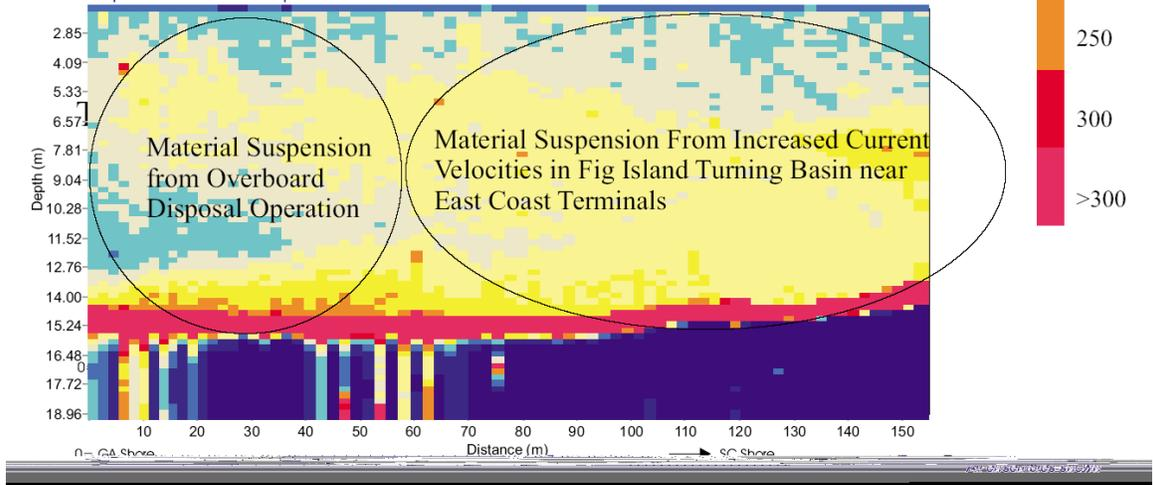
**Figure 7. Example SEDIVIEW output showing containership plume (top) and a comparison of overboard disposal with strong river currents.**
