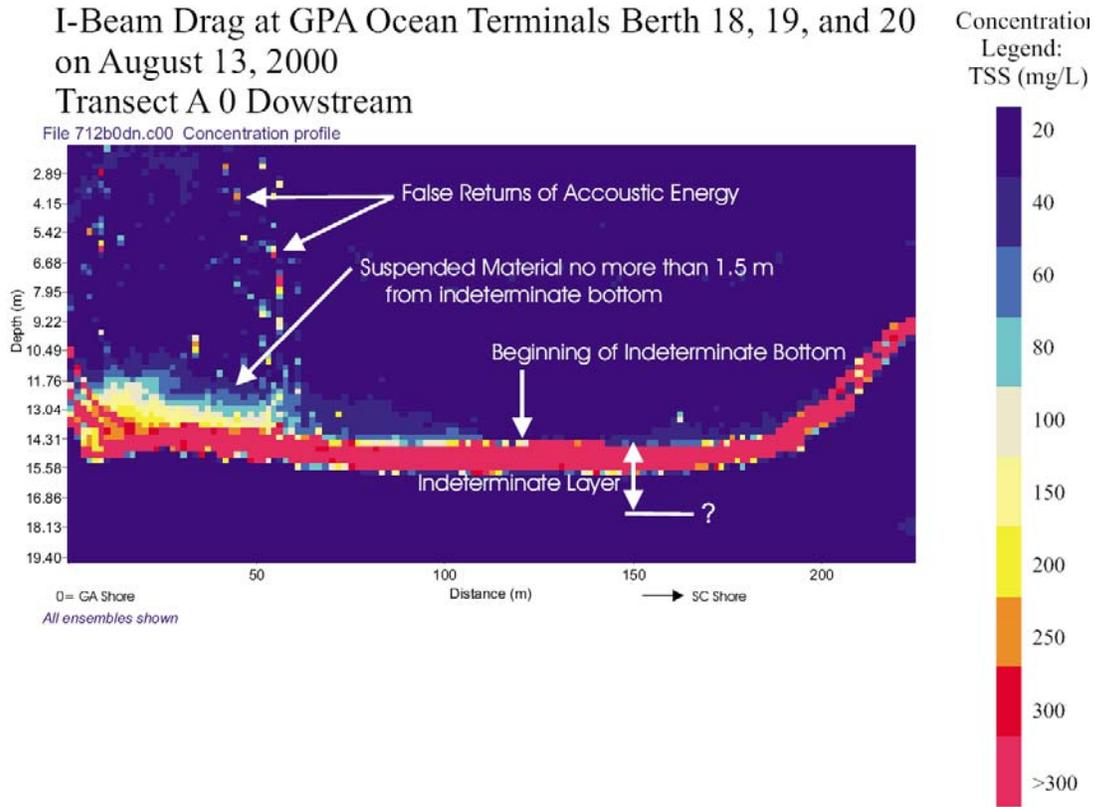
**Figure 5. Example SEDIVIEW output plot of I-Beam dragging. This is a cross-section view of the river.**
